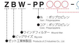
●ろ過精度 (μm) Filtration accuracy (μm) 0.5, 1, 3, 5, 10, 25, 50, 75, 100, 150, 200
